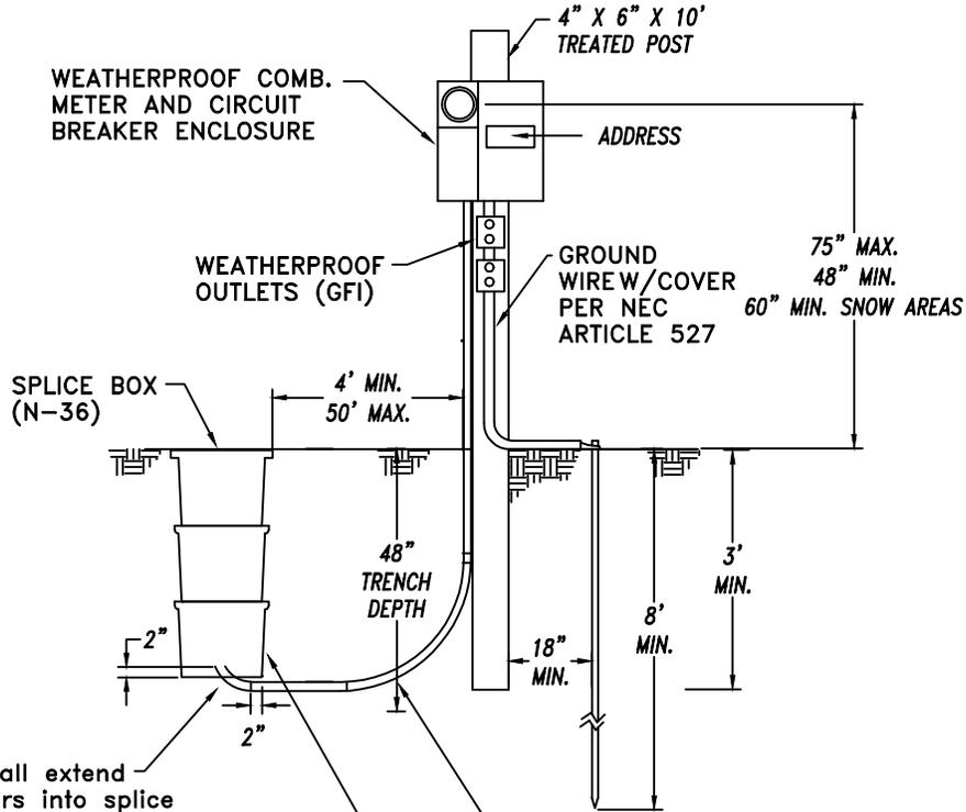
Customer shall extend his conductors into splice box a minimum of 48". LU will make connections.
