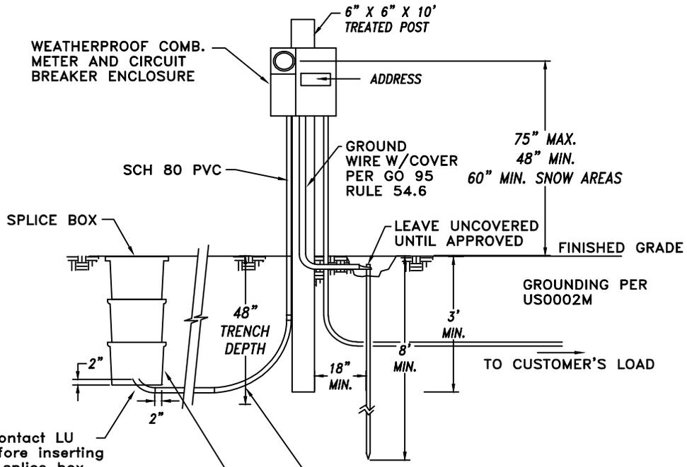
CAUTION: Contact LU inspector before inserting conduit into splice box. Conduit will curve up into the bottom of the box. Box will not rest (touch) on conduit(s).
