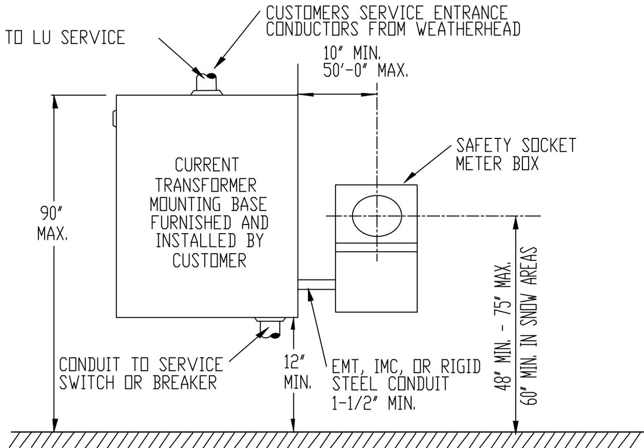
For single overhead irrigation service which is to be metered using current transformers, the customer shall furnish, install, own and maintain a separate current transformer cabinet and safety socket meter box and required service entrance conductors, conduit and weather head to the point of attachment of LU's overhead service. The bussed current transformer cabinet is also acceptable for this application. Equipment shall conform to EUSER Committee Standards.
