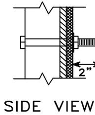
5/8" BOLT, WASHER AND BACKING PROVIDED BY BUILDER, EXTENDING MIN. 2" FROM FACE OF SIDING
